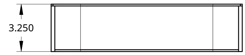
BENT PIECE (AFTER BENDING) (1/4" PLYWOOD) *kerf cuts not shown
